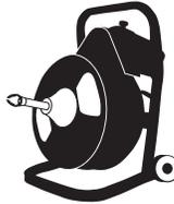
**IMPORTANT** Use a drain machine to remove build up inside pipes. Clean as far into the line as possible, up to 25 feet, to remove debris.
